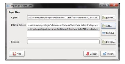
Clicking on **Import** starts the process of importing data. Leapfrog will display a series of windows, one for each file, and will attempt to match the data found in the files with the columns expected, based on the header row in each file.
