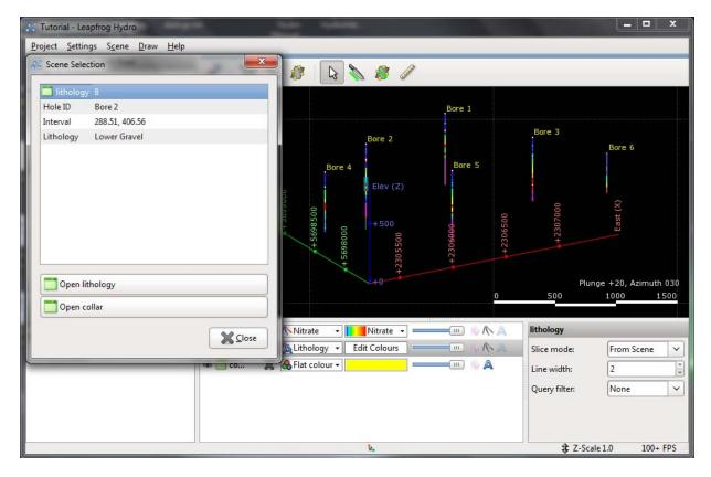
Click the **Open lithology** and **Open collar** buttons to go directly to the corresponding tables, where the selected data segment will be highlighted. In this example, the lithology table is displayed:
