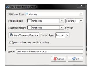
The **GIS Vector Data** drop-down list displays all vector data in the project that can be used to create a new contact surface. If the data you wish to use does not appear in the list, ensure that it has been imported into the project.
