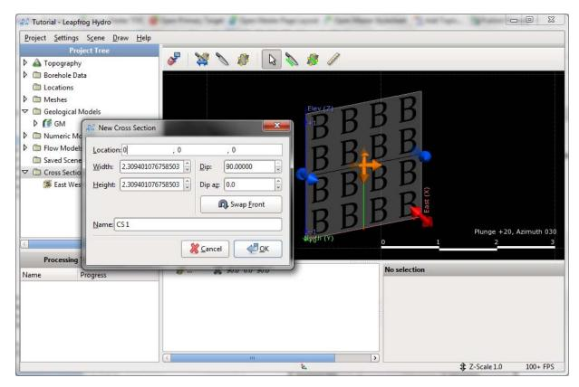
The back of the cross section is marked with the letters B, while the front of the cross section is marked with Fs.
