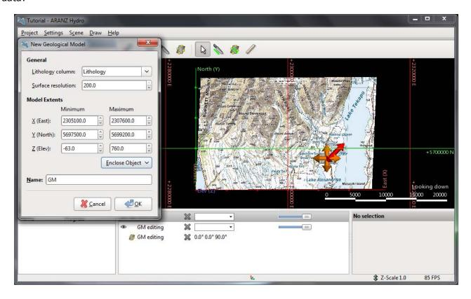
The **Surface resolution** is also set in this window. A lower value will produce more detail, but calculations will take longer. The advantage of Leapfrog over many other geological modeling products is that the surface resolution can be easily changed.
