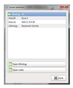
You can open the relevant lithology and collar tables by clicking on the **Open lithology** and **Open collar** buttons, with the selected segment highlighted. This is useful when, for example, displaying borehole data in the scene makes it apparent that the data for that borehole is incorrect.
