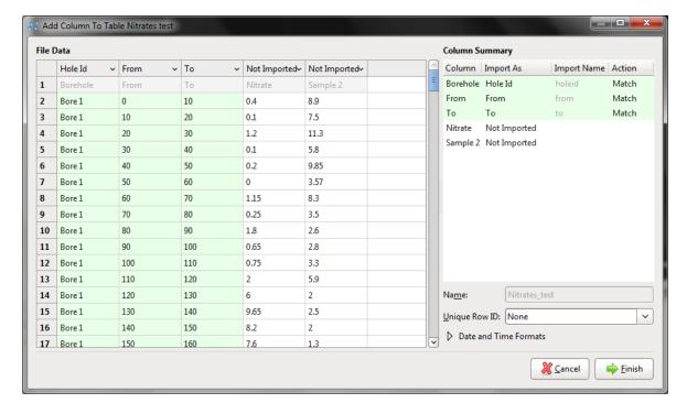
Select as many columns to import as required and assign the appropriate data type. Before finishing, check the **Column Summary** to ensure that the correct information will be imported:
