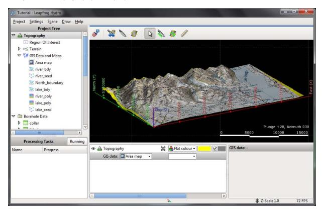
Now that the terrain is defined, maps will be automatically draped over the topography. The imported mesh is stored under the **Terrain** object. A copy is also stored in the **Meshes** folder. The next step is to add information about land use. See <u>Adding Information About Land Use</u>.
