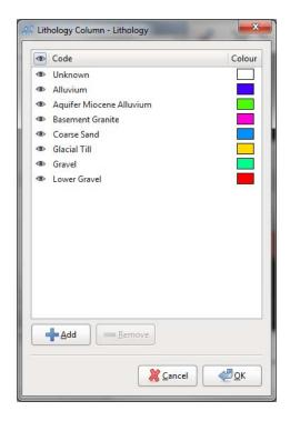
All the lithologies found in the specified column in the borehole data have been assigned colors. An additional lithology also appears in the list, called "Unknown". This is automatically added to the list of lithologies so that any unknown volumes generated when the geological model is built can be highlighted as this lithology.
