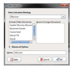
Select the lithology that will remove existing materials from the **Select intrusion lithology** drop-down box, then select the options required. Click **OK** to generate the new contact surface.
