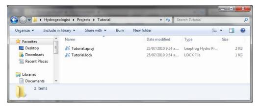
The Tutorial.lock file is created when the project is opened and closed when the project is closed. Later, once you have added borehole data to the project, there will be an additional file, ending with .apbd. The .apbd file contains all the borehole data imported into a Leapfrogproject.
