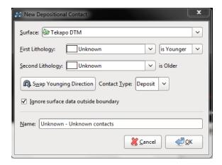
The **Surface** drop-down list displays all the surfaces in the project that can be used to create a new contact surface. If the surface you wish to use does not appear in the list, ensure that it has been imported into the project.
