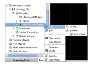
You can add points data, meshes and GIS vector data to any lateral extent. Select the required option and Leapfrog Hydro will display a list of the data that can be used for the lateral extent.
