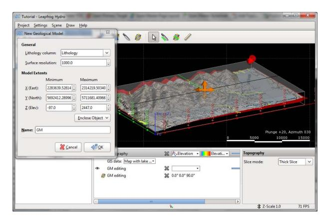
This window lets you set a basic rectangular set of model extents aligned with the south/north and east/west axes. There are three ways to do this:
