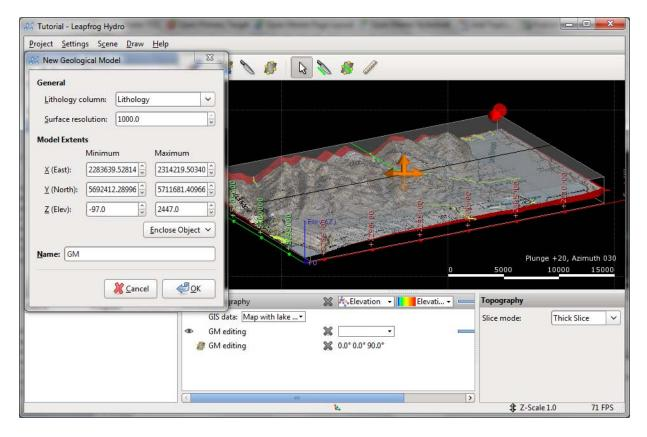
This window lets you set a basic rectangular set of model extents aligned with the south/north and east/west axes. It is possible to describe irregular-shaped model extents, which is discussed further
