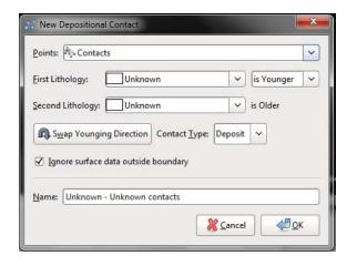
The **Points** drop-down list displays all points data in the project that can be used to create a new contact surface. If the data you wish to use does not appear in the list, ensure that it has been imported into the project.
