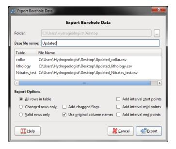
The list shows the files that will be created, one for each data table. Choose a folder where the files will be saved, then enter a **Base file name**, which will be added to the front of each file name. For example, entering "Updated" for the **Base file name** results in files called <code>Updated\_collar.csv</code>, <code>Updated\_lithology.csv</code> and <code>Updated\_Nitrates\_test.csv</code>.
