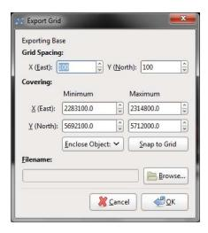
Enter a name for the new elevation grid file and click **Browse** to choose a location. Choose the **Grid Spacing** and **Covering** properties, then click **OK** to save the grid.
