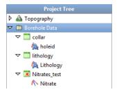
When there are errors in the data, the relevant table will be marked with a red X. See <u>Correcting</u> <u>Borehole Data Errors</u> for more information on fixing data errors.
