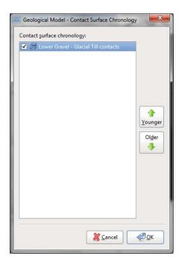
Tick the box to add the Lower Gravel – Glacial Till contact surface to the chronology, then click **OK**. This results in Leapfrog generating the first two volumes, which are added to the **Output Volumes** object:
