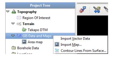
Navigate to the folder that contains GIS data files and import the files, one at a time. For each file, the **Import GIS Vector Data** window will be displayed:
