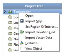
You can also right-click on objects within the top-level objects to view more information on that object or carry out actions specific to that object. For example, right-clicking on a table of imported borehole data reveals a menu showing possible actions:
