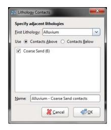
The **Contacts Above** and **Contacts Below** lists display the number of contacts that exist in the borehole data between the **First Lithology** and those it comes into contact with.
