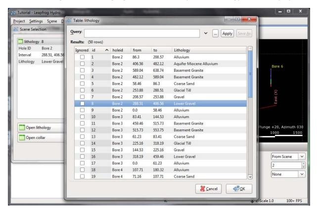
In this table, you can change any entry by clicking on the row, then on the value. This is useful when the three-dimensional display of the data has made errors apparent. Edited data can be exported from Leapfrog.
