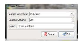
The **Surface to Contour** dropdown list contains all the surfaces in the project. Select the surface to use for the new contour and adjust the **Contour Spacing**, if required. Click **OK** to generate the surface.
