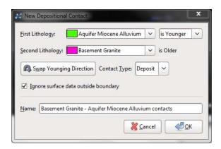
Because the process for generating a depositional contact surface is similar to that for generating an erosional surface, you can change the **Contact Type**.
