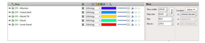
The icons displayed for the **Slicer** object correspond to the different menu options in the **Scene > Slicer** menu. Finer controls over the slice properties are also available in the properties frame.
