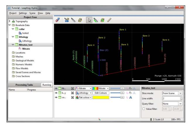
The appearance of the displayed data can be changed by changing the properties of the object in the shape list. For example, when the data is first add to the scene, the collars are displayed as small points:
