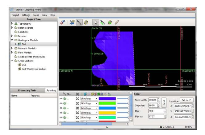
Next, right-click on the **Cross Sections** object and select **New Cross Section From Slicer**. The **New Geology Section** window will be displayed:
