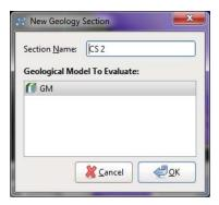
A list of the geological models created in the project is displayed in the **Geological Model To Evaluate** list. Select the model required, enter a **Section Name** and click **OK**. The new cross section will be created and added to the **Cross Sections** object. Display it by clearing the scene, then adding the cross section to the scene. The cross section will appear in the scene:
