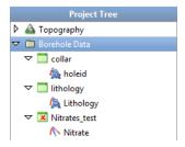
The Nitrates\_test object has an X across is because there are errors in the data. See <u>Correcting</u> <u>Errors in the Data</u>.
