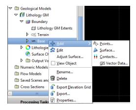
You can add points data, meshes, lithology contacts and GIS vector data to the base. Select the required option and Leapfrog Hydro will display a list of the data that can be used for the base. You can edit the base and adjust the surface.
