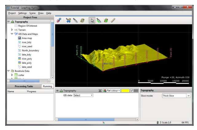
The **Topography** object in the shape list provides additional controls that can be used to change the way the topography is displayed and highlight features of interest. For example, selecting an imported map from the dropdown list results in it being displayed draped onto the terrain:
