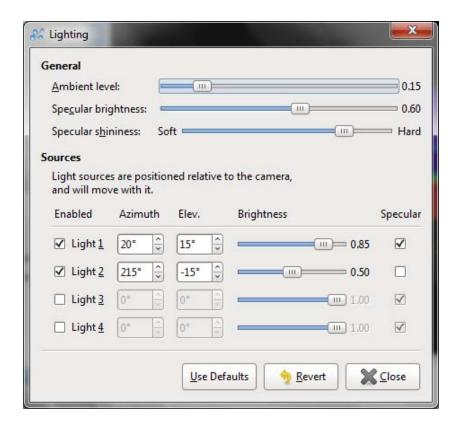
The **Ambient level** setting determines the overall brightness of the scene.
