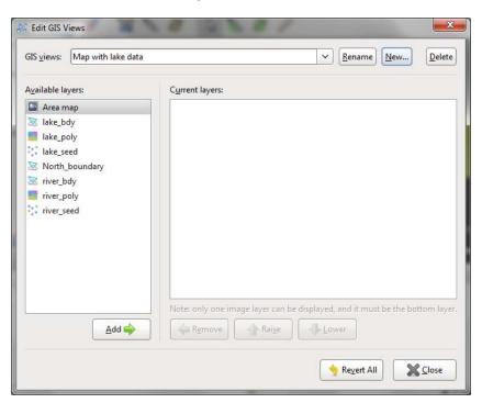
To add a layer to the view, click on it, then click the **Add** button. You can change how the different layers are displayed using the controls in the **Current layers** list and change the order of layers using the **Raise** and **Lower** buttons.
