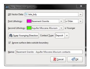
Because the process for generating a depositional contact surface is similar to that for generating an erosional surface, you can change the **Contact Type**.
