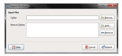
Appending borehole data is similar to importing the original collar and interval tables (see <u>Importing Borehole Data</u>). Leapfrog will ask you to specify the file location, and then will display the data in the file in the **Import Tables for Appending** window.
