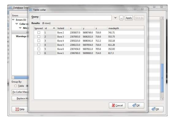
The maximum collar depth specified for Bore 4 is 332.18, which conflicts with the nitrate data collected for Bore 4.
