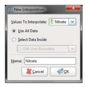
If more than one column of numeric data has been imported, the different columns can be selected from the **Values To Interpolate** dropdown list.
