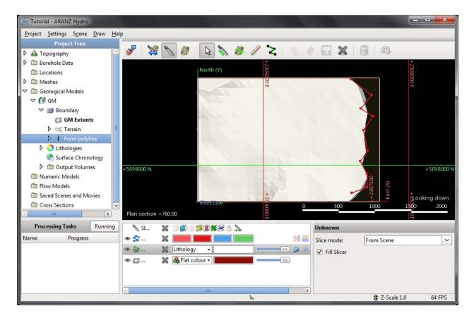
However, the polyline object remains in the scene. Remove it and the **Slicer** from the scene by clicking the X next to each object in the shape list:
