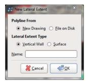
Make sure **New Drawing** and **Vertical Wall** are selected, then click **OK**. Click on the **Draw lines** icon, then on the **Slicer** tool in the shape list.
