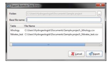
The list shows the files that will be created, one for each table that contains errors. Choose a folder where the files will be saved, then enter a **Base file name**, which will be added to the front of each file name. For example, entering "errors" for the **Base file name** results in two files called errors\_lithology.csv and errors Nitrates test.csv:
