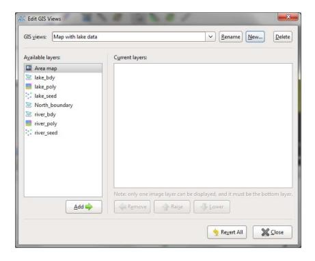
Add the required layers to the **Current layers** box and use the **Raise** and **Lower** arrows to arrange the layers.
