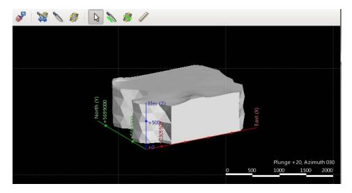
Now that two new extents have been created, double-click on the **Boundary** object to open the **Geological Model Boundary** window. The two lateral extents now appear in the **Lateral Extents** list and can be added to or removed from the model by ticking the box.
