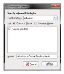
Best practice is to build the geological model from top to bottom, so for this tutorial, build the "Lower Gravel – Glacial Till" contact surface first. To do this in one of two ways:
