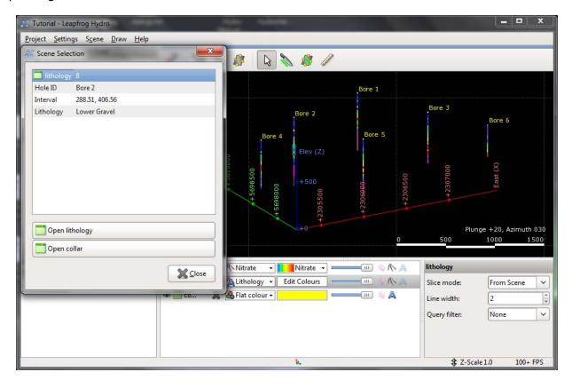
These scene selection windows also provide access to the data tables behind the individual data points. For example, in the screen above, the **Open lithology** and **Open collar** buttons open the tables relevant to the selected segment:
