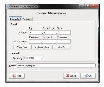
In the **Interpolant** tab, you can define the directional trend (anisotropy) and set the accuracy of the interpolation. For example, if the resulting surfaces weren't as faithful to the data as required, the accuracy could be reduced.
