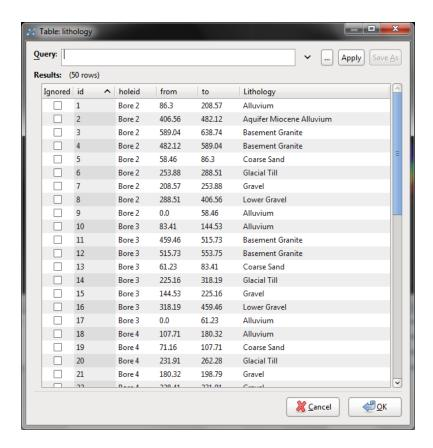
You can also open a data table by clicking on a segment displayed in the scene. For example, clicking on a borehole segment in the scene will display the **Scene Selection** window and detailed information about the segment clicked on:
