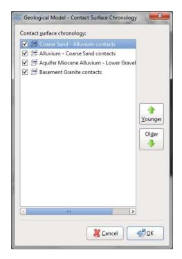
The **Contact surface chronology** list displays all the contact surfaces that have been generated. To add a surface to the surface chronology, tick the box for it. Use the **Younger** and **Older** buttons to change the order in which surfaces appear in the chronology.
