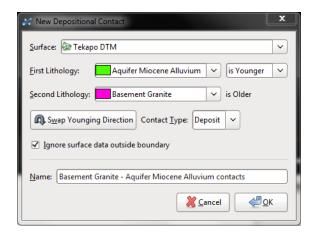
Because the process for generating a depositional contact surface is similar to that for generating an erosional surface, you can change the **Contact Type**.
